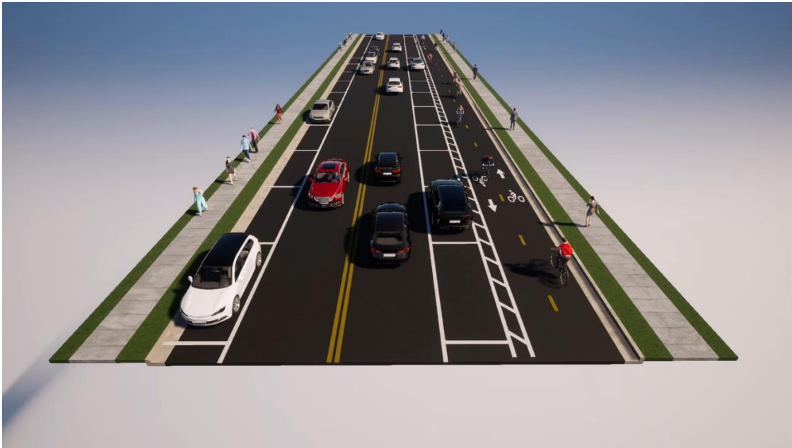
Figure 6: Conceptual Depiction of Two-Way Street with On-street Parking and Two-Way Cycle Track
